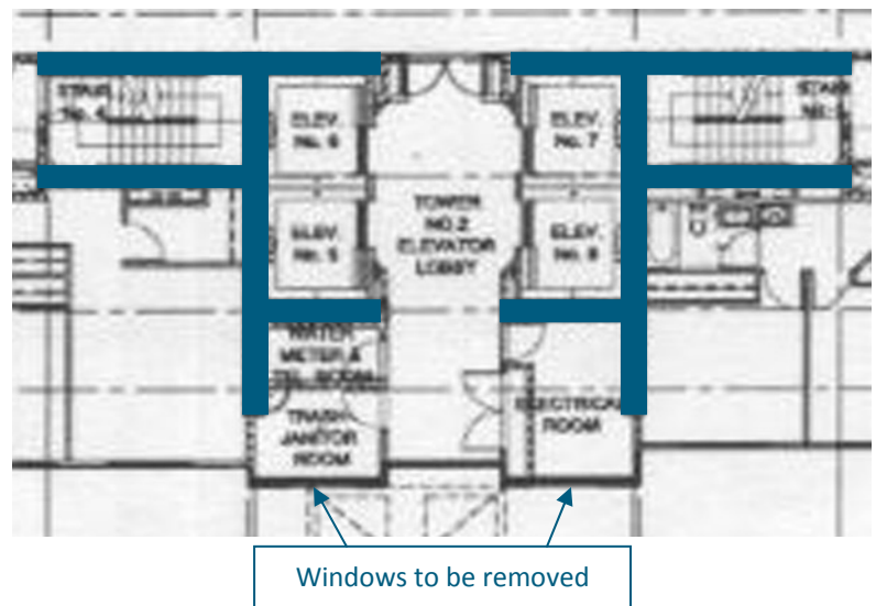
Figure 17 – Original Shear Wall Locations
